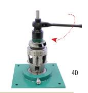
5 Place TORQUE TESTING NUT and use TORQUE WRENCH with INSERT to tight at correct torque (clockwise)
