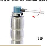
Loosen with Allen Tool, remove from Fixture Seat. Remove 4" Jig with Allen Tool from Assembly
