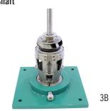
4 Use WRENCH FOR IMPELLER NUT to tighten (clockwise)
