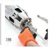
20 Pull out SHAFT using DEPTH TOOL
