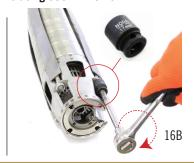
Use TORQUE WRENCH and FIXTURE FOR STRAP to tight at correct torque (clockwise)
